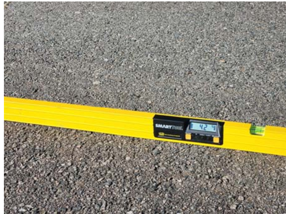
Figure 16 – Sta. 0+50 pavement walkway profile slope of 4.2%.
