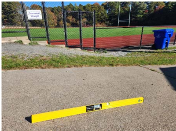
Figure 17 – Concrete walkway profile slope
