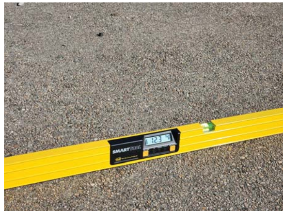
Figure 18 – Concrete walkway profile slope of 12.3%.
