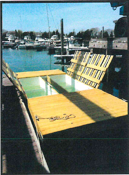
Figure 1. Floating downweller. The shellfish grown in the Pocasset River will be grown under the existing docks in stacked trays like in the pictured system.
