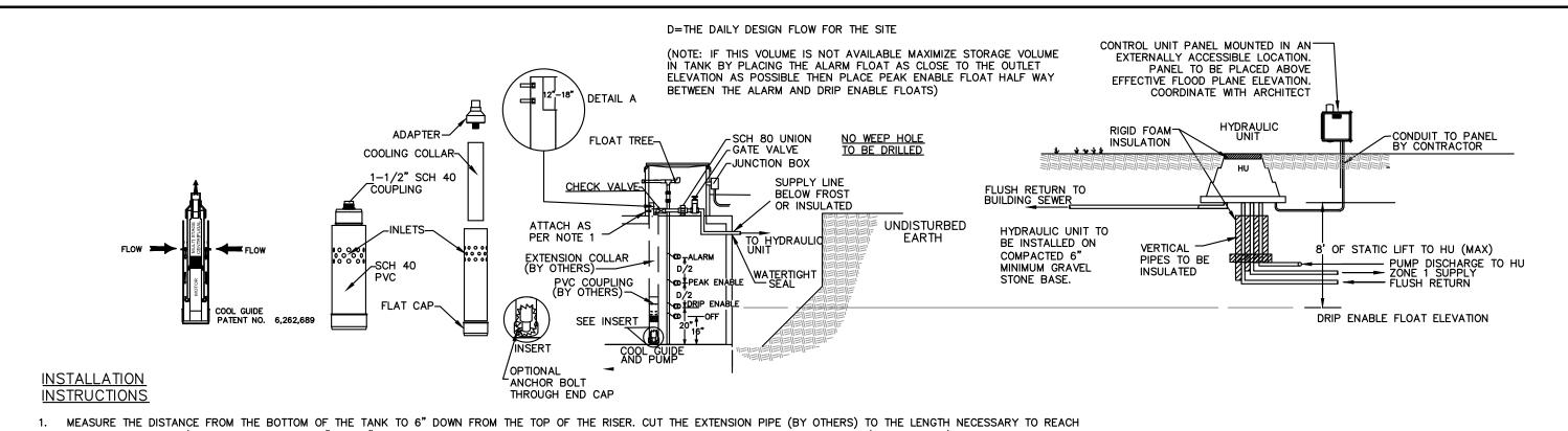
THIS HEIGHT. CUT 1/2 OF THE PIPE DOWN 12" TO 18" AWAY FROM THE TOP OF THE PIPE FOR PUMP DISCHARGE PIPE AND ATTACH TO RISER (SEE DETAIL A). GLUE THE EXTENSION COUPLING (BY OTHERS) TO THE EXTENSION PIPE AND TO THE COOL GUIDE.
