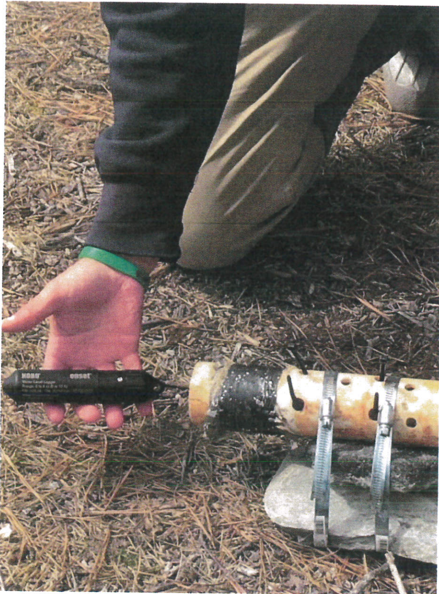
Figure A15: Photo of one Onset HOBO Water Level Logger and the instrument housing; vented PVC housing, large stone anchor. HOBO logger inserts into PVC housing and fastens with zip ties.
