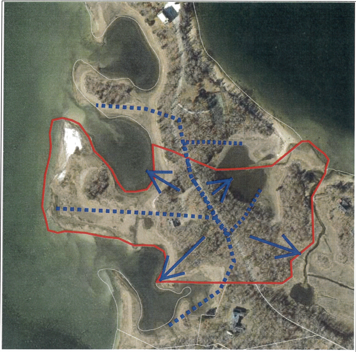
Figure 3 - Conceptual Groundwater Flow Patterns
