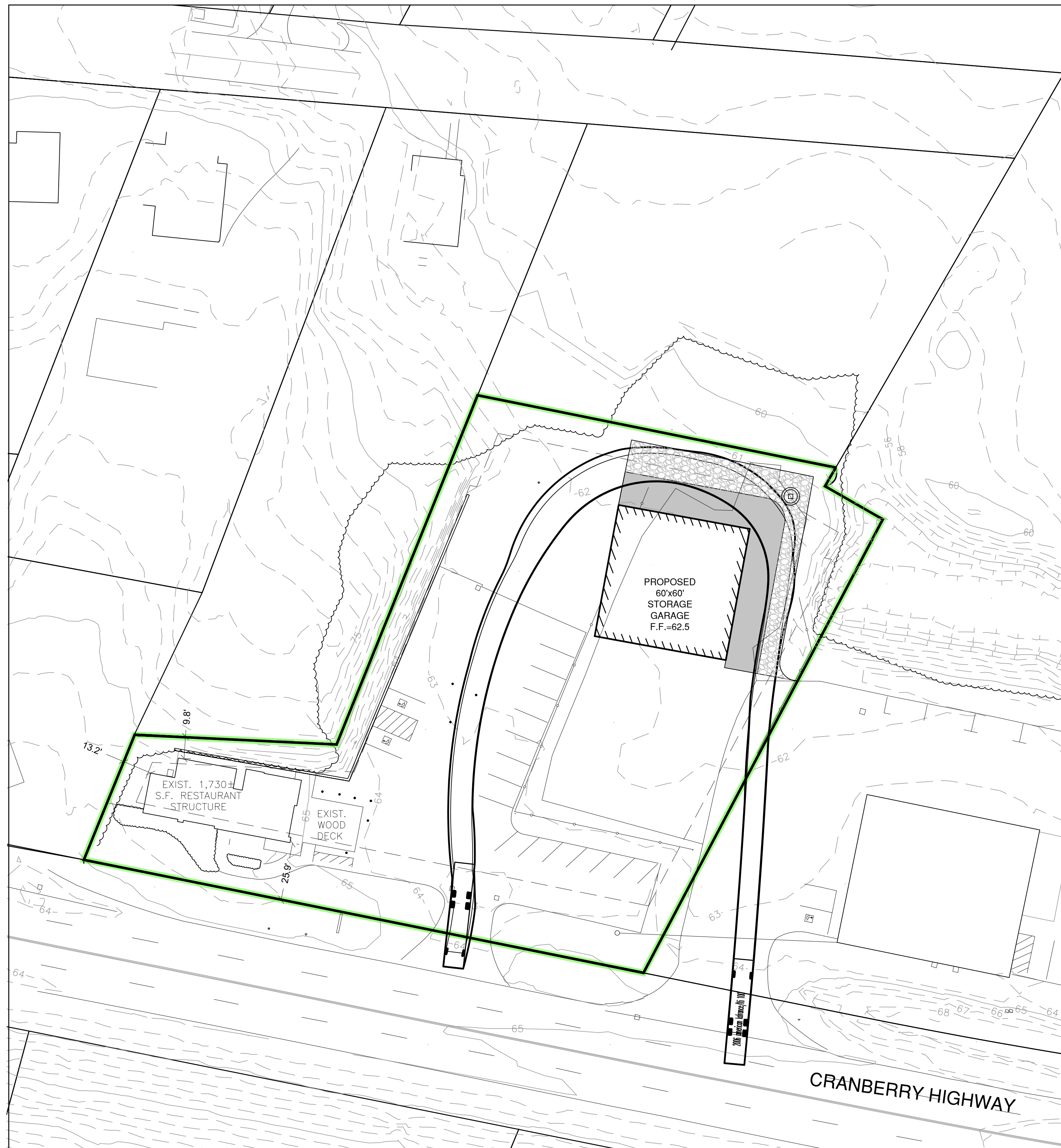
TRUCK TURNING PLAN SCALE: 1"=30'
