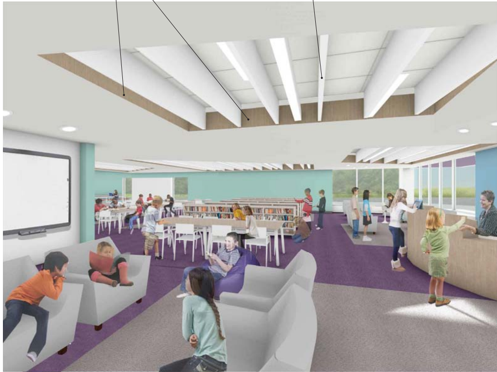
Wood Veneer on Vertical Face of Soffit
