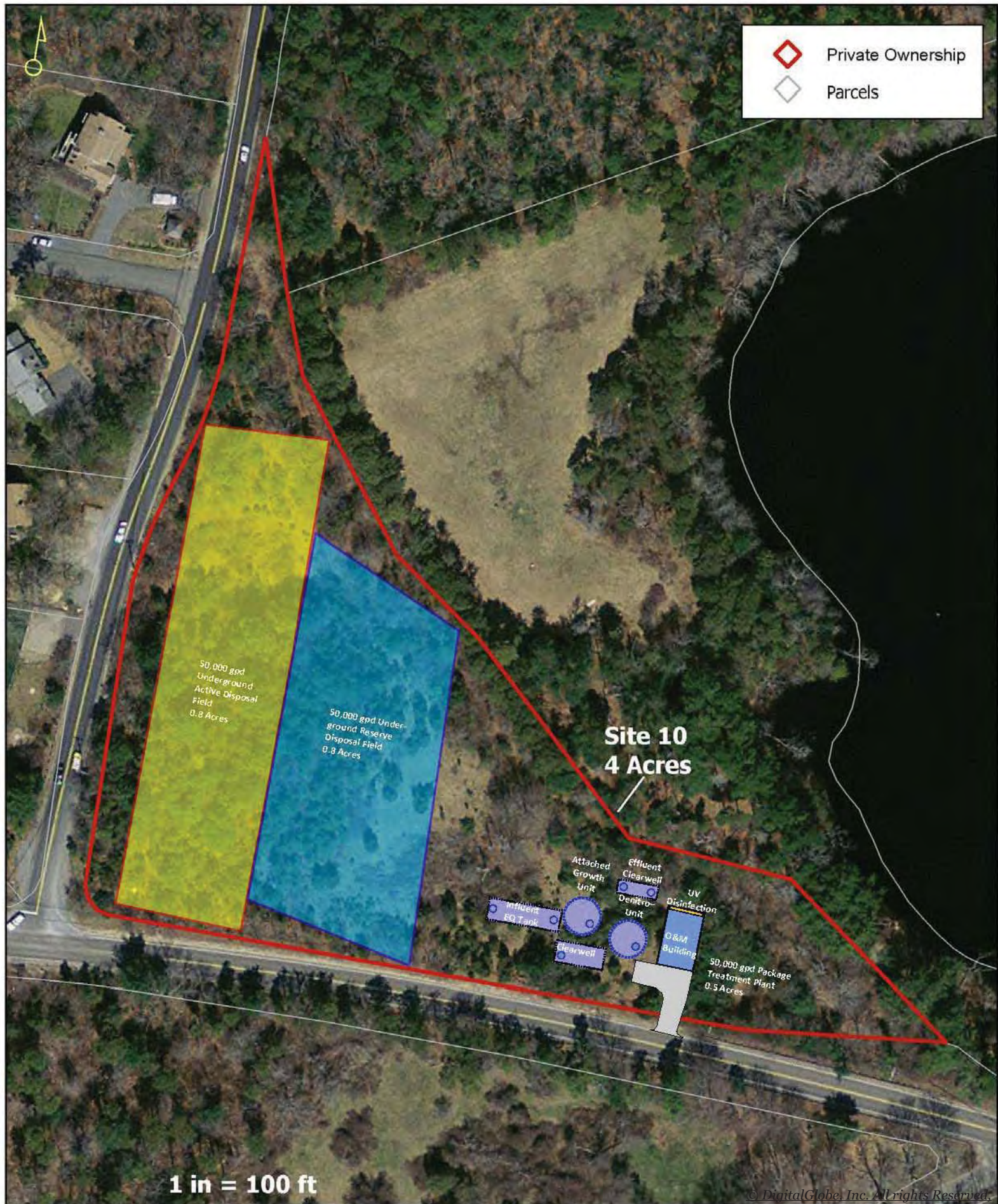
FIGURE 24. OPTION OF HIDEAWAY VILLAGE WASTEWATER TREATMENT- 50,000 GPD PACKAGE PLANT AND SUBSURFACE DISPOSAL (NOT RECOMMENDED - FINANCIALLY INFEASIBLE)
