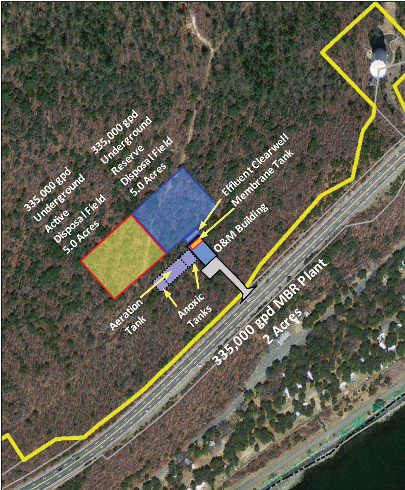
FIGURE 23. CLOSEUP OF PREFERRED OUT OF DOWNTOWN OPTION – 335,000 GPD MBR TREATMENT PLANT AND SUBSURFACE WASTEWATER DISPOSAL
