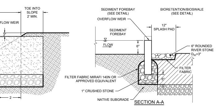
1. KEY GRANITE CURBING INTO THE FOREBAY SIDE SLOPES AND EXTEND A MINIMUM OF 2' TO PREVENT FLOW FROM DIVERTING THE CHECK DAM
